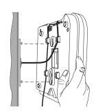
3. Place the Base Unit on the posts of the wall plate and push down until it's firmly seated.
